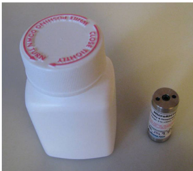
Fig. 1. Picture of 75-cc HDPE bottles and data loggers used in this study
